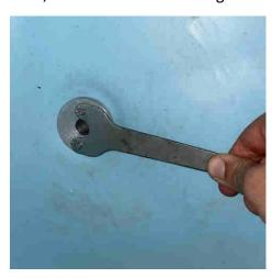
**Step 6:** At the lower outside part of the bin, we will place the reinforcing plate. We insert the thread of the protruding cover into the hole of the reinforcing plate.
