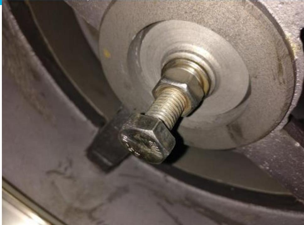
**To remove the bearing, you can tighten the lower screw, making it come out of the bowl. To mount, simply force down the entire shaft and place the screw without tightening too much.**
