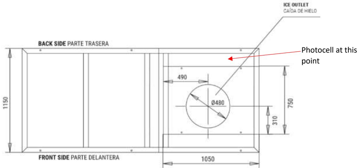
Ice maker underside, with ice outlet dimensions
