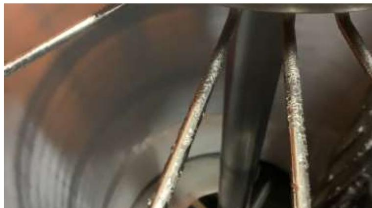
*Evaporator, with difference between rings, after adjustment*
