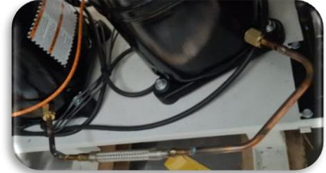
**13.** Place the nuts that we have removed in point 5. It's very important to place the joints correctly.
