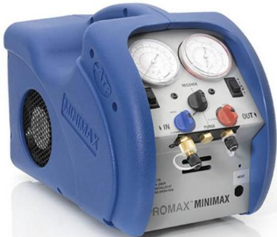
3. Connect the gas recycler to empty the machine.
