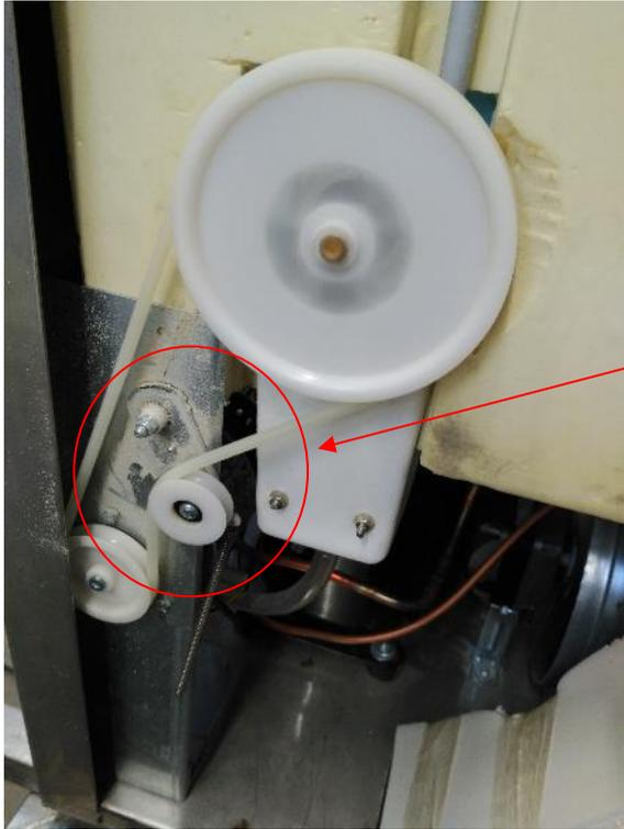
In the MP145 remove the tensioner, removing the screw and removing the anchor plate with tensor
