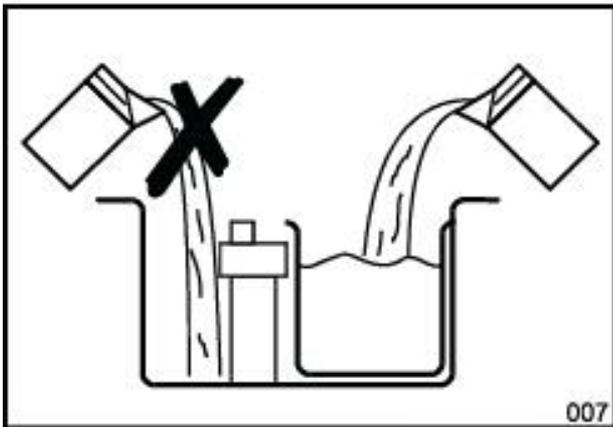
During the washing step the pump can be working constantly, but always with water in the cream bin. **The unit should not work without liquid to prevent damaging the pump.**
