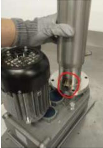
7. Place the auger into evaporator
