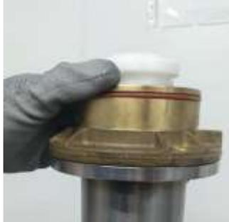
16. Screw the kit extruder to evaporator at correct position in order to screw the ice exit plastic cover.
