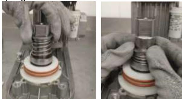
Fit Seeger washer into the shaft slot
