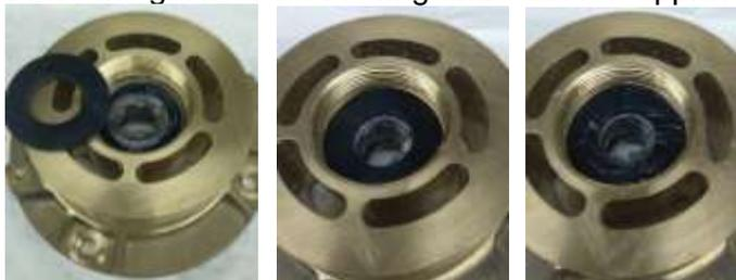
Place the O-ring at external extruder slot and add NSF approval grease
