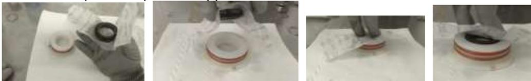
Add NSF approval grease to the two O-rings in order to improve the evaporator assembly
