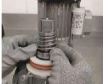
Place the washer over spring and push it downwards in order to compress the spring
