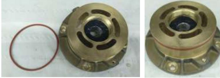
14. Screw the ice breaker to extruder with the hand.
