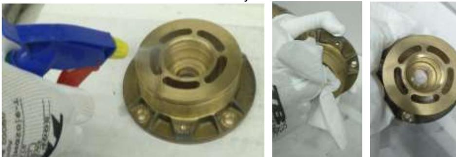
Place the small o-ring into extruder slot at the bottom and add NSF approval grease on it
