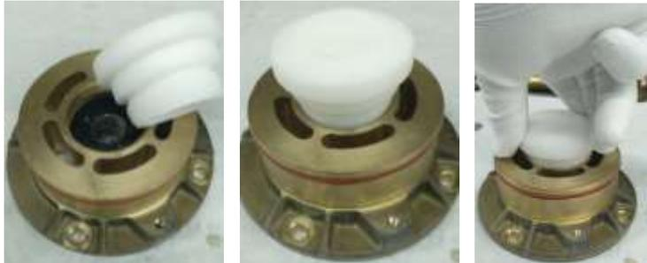
Tighten the ice breaker with a tool like image (tool used to change the disc of Angle Grinder machines)
