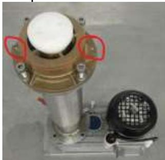
17. Place and screw ice exit plastic part to extruder, place evaporator insulation, place ice exit plastic cover and attach plastic cover with O-ring.
