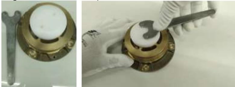
15. Place the kit extruder on top evaporator.
