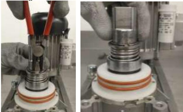
5. Place evaporator on gearmotor
