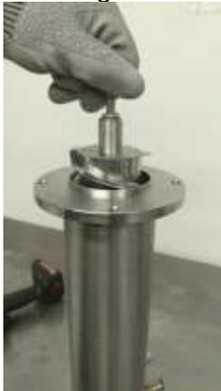
The auger is at the correct position if it is above evaporator (0,024 inch máx (0,6 mm max) )
