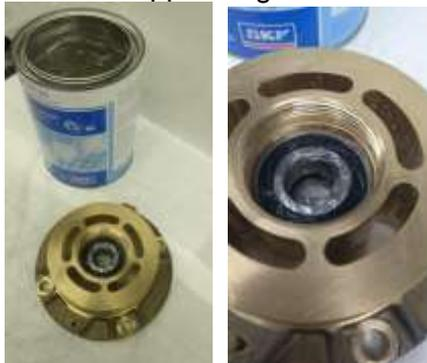
13. Place the gasket over bearing and add NSF approval grease on its top surface
