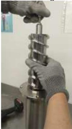
8. Turn auger in order to fit to gearmotor shaft
