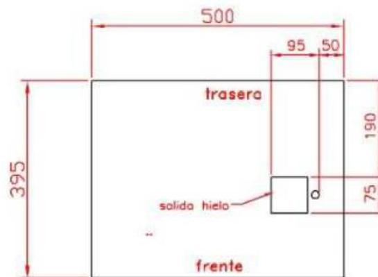
The hole in the top cover of the ice bin must be wider than 30 mm next to the bounded area
