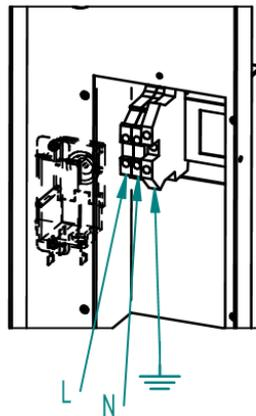
*Terminal connector to supply electrical power to the remote condenser, located behind the metallic cover.*
