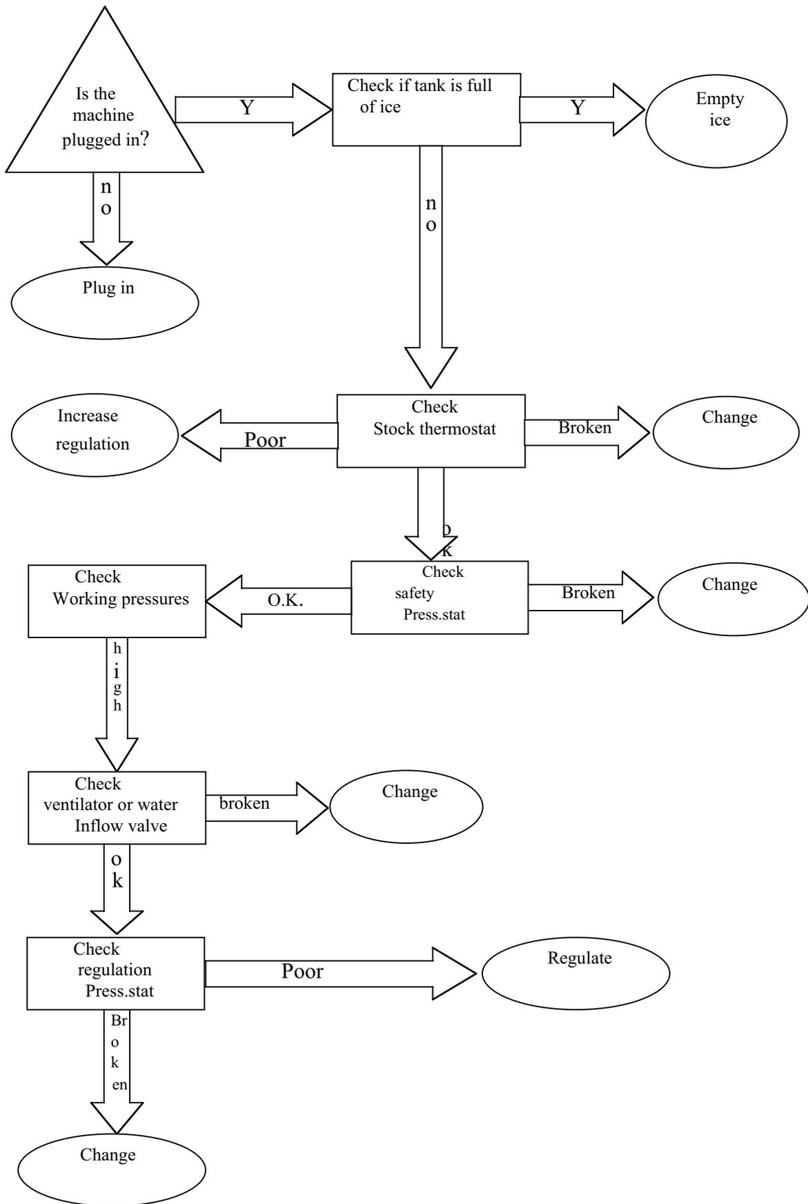
7.2. The Machine is Operating but Fails to Make Ice
