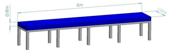
The volume of ice required is 6 m x 1.1 m x 0.18 m = 1.19 m3 of ice
