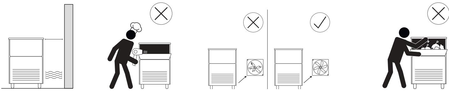
**EN.** In case of refrigerant leakage:
