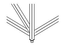
Note: The legs should not exceed a total height of 54 mm.
