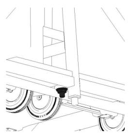
Place the bent end onto the connection at the bottom of the ice storage bin by force-fitting. The other part will go to an outside drain.
