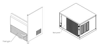
Clean condenser using a vacuum cleaner, soft brush or low pressure air. Clean from top to bottom, not side to side. Be careful not to bend the condenser fins.
