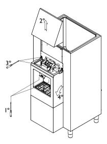
The rest of the panels form a unique block. First unplug all the connections of the electrical parts that are mounted on it (LED light, water button, etc...), then unscrew the 2 screws (see figure). The block can be removed by tipping it slightly and extracting it upwards, to release it from the 2 bottom tabs.
