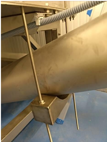
Cradle for endless support exit. If necessary, place a clamp.
