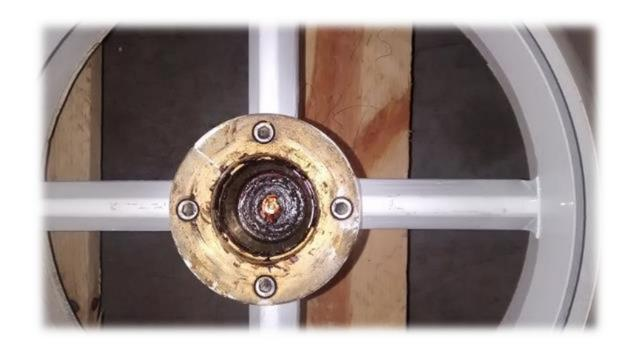
After removing the main shaft, we will have access to the lower conical bearing ring.
