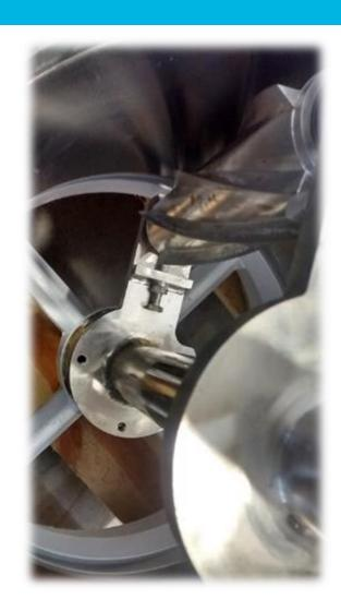
Once the water baffle is removed, we find the main cutter.
