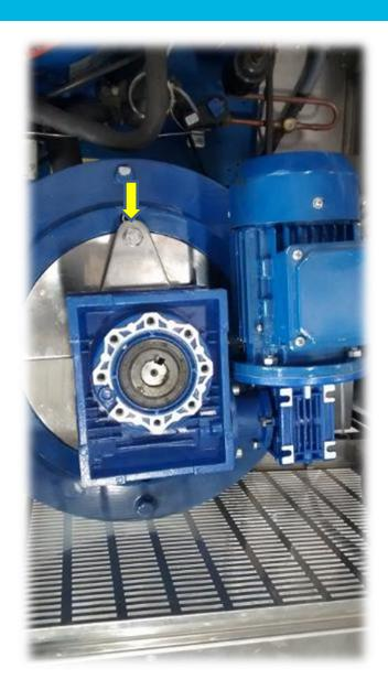
Remove the screw indicated in the image. Once removed, the gear motor can now be pulled up.
