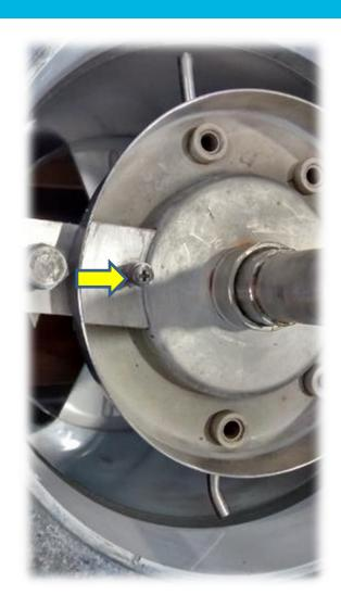
Once the upper ring is removed, we find the water distributor tray. To remove it, you have to remove the screw indicated in the image, it has silicone between axle and tray. The shaft can be removed without removing the tray.
