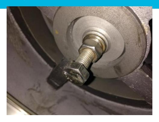
To remove the bearing, you can tighten the lower screw, making it come out of the bowl. To mount, simply force down the entire shaft and place the screw without tightening too much.
