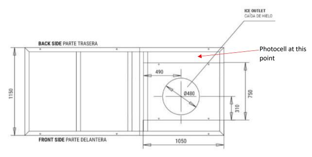
Ice maker underside, with ice outlet dimensions
