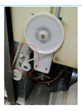
Check that the pulleys are in the same plane, level, if they are in different planes, there is a greater effort in the belts and they break or get loose out of the wheel. Can be checked visually or with level.
