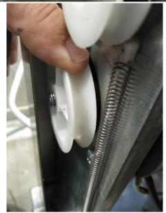
If the belt deteriorates, white dust will be seen from the belt rubbing on the turbine motor support.
