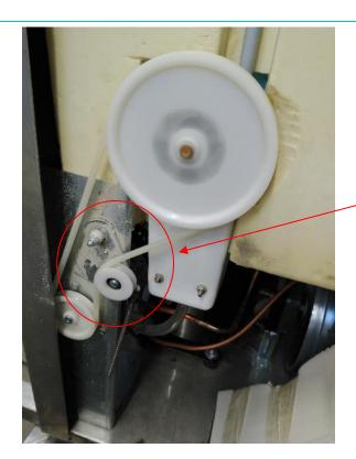
In the MP145 remove the tensioner, removing the screw and removing the anchor plate with tensor
