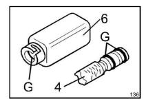
When dismantling parts for washing, regularly check that gaskets [G] are intact and replace them if damaged or dilated.
