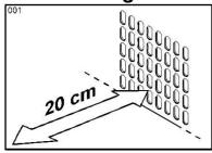
Place the machine on a flat and steady surface.
