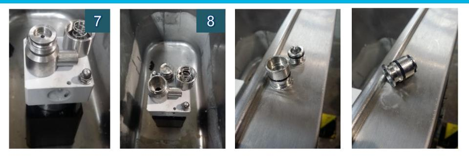
7. Dismantle the air regulator pulling it upwards. Remove the regulator switch turning it counter clockwise.
