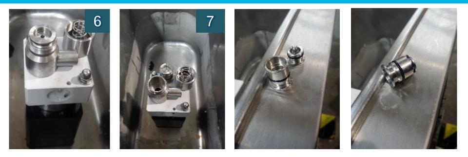
6. Dismantle the air regulator pulling it upwards. Remove the regulator switch turning it counter clockwise.
