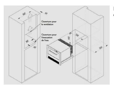
[Ventilation opening/ Water drainage opening]
