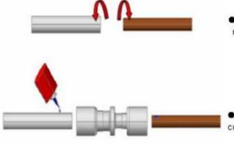
clean the tube ends with abrasive mat in a rotational motion around the tube
